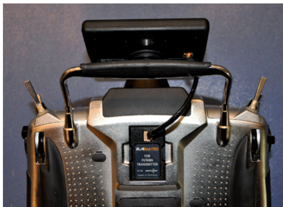
weatronic Adaptermodul am Futaba T14MZ Sender
