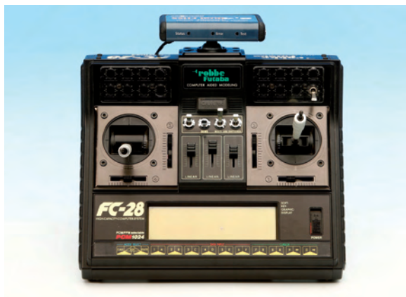
weatronic Sendemodul am Futaba FC-28 Sender
