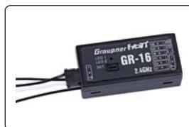
Connect the adapter lead to the socket on the left-hand end of the receiver, as shown in the illustration. This socket is also polarised; note the small chamfer on one edge. Never use force - the plug should engage easily and fully.
