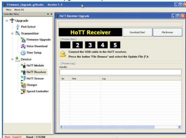
Under „Port Select“ select the correct COM port „Silicon Labs CP210x USB to UART Bridge“, i.e. the one to which the USB lead is connected.
